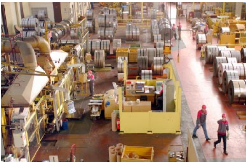
THE COLD ROLLING MILL at Imphy where coils of low-expansion nickel alloy are produced.
